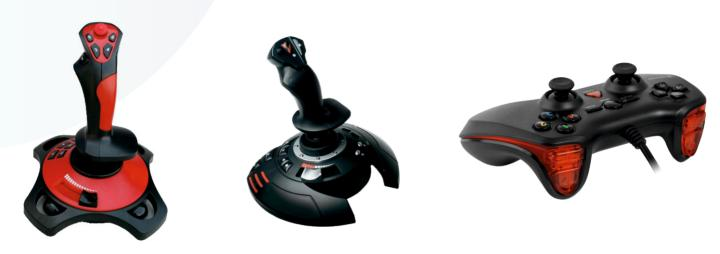
When you press the button on the joystick and move the stick, you instruct the computer to play as you wish, so it is an input device.
